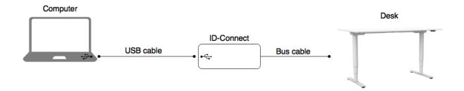
Figure 1 - The ID-Connect connected to the computer with an USB cable and to a desk with a bus cable.
